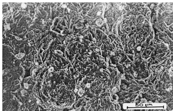
Fig. 4. Scanning electron micrograph of fresh Pb-Co 3 O 4 anode.
